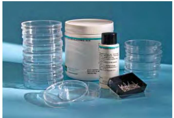
Make your own silicone dissection pads easily and quickly. Mix the 2-part silicone right in the plastic petri dishes and allow to cure 24 hours at room temperature. Kit includes enough silicone to prepare 20 dishes.
