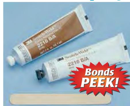
Probably still the best epoxy for bonding plastic, often used as the benchmark for testing the binding strength of other adhesives. The slightly rubbery texture also makes it less easy to break off. *It is the only epoxy known that can bond PEEK.* Color: gray. Cures at room temperature.
