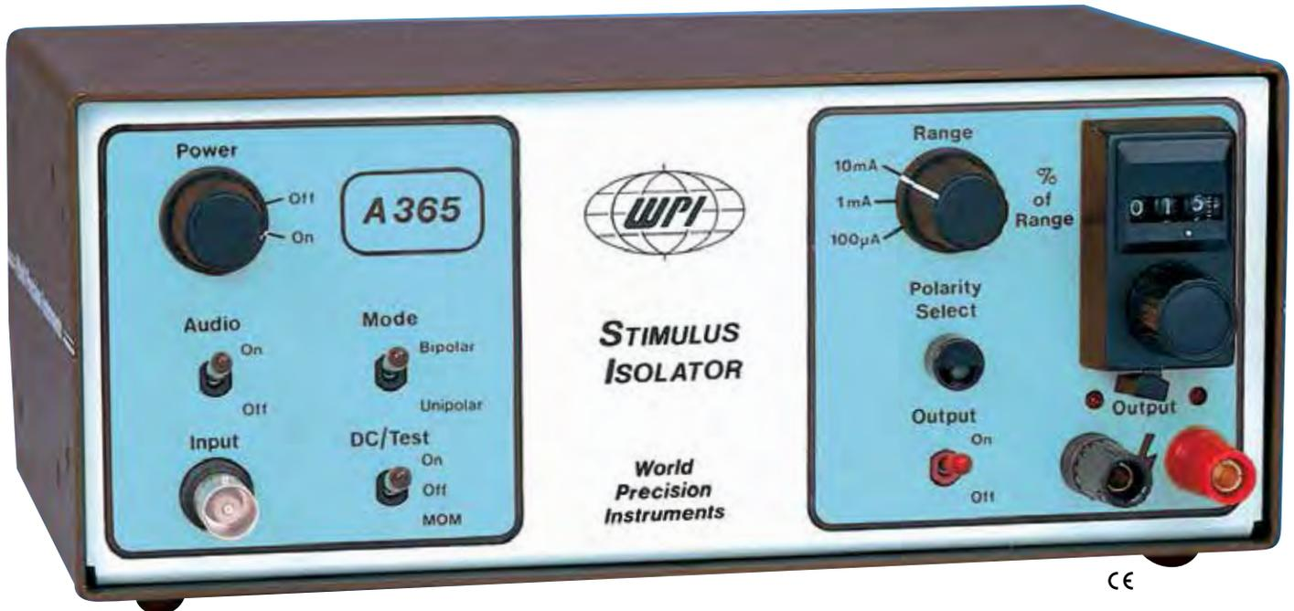
**Model A365** includes the same features and specifications as A360 but with the added capability for automated bipolar pulsing for zero net charge on biological preparations.
