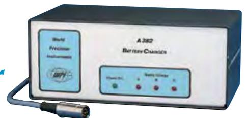
An innovative three-step charger, A382 employs fast, medium, and trickle charges at a safe, low current, greatly extending battery life. After a fast initial phase, the charger automatically switches to a constant voltage mode. When charging is complete, the charger switches to the trickle-charge mode. LED lamps indicate charging status. (For use only in charging batteries installed in the A385.)
