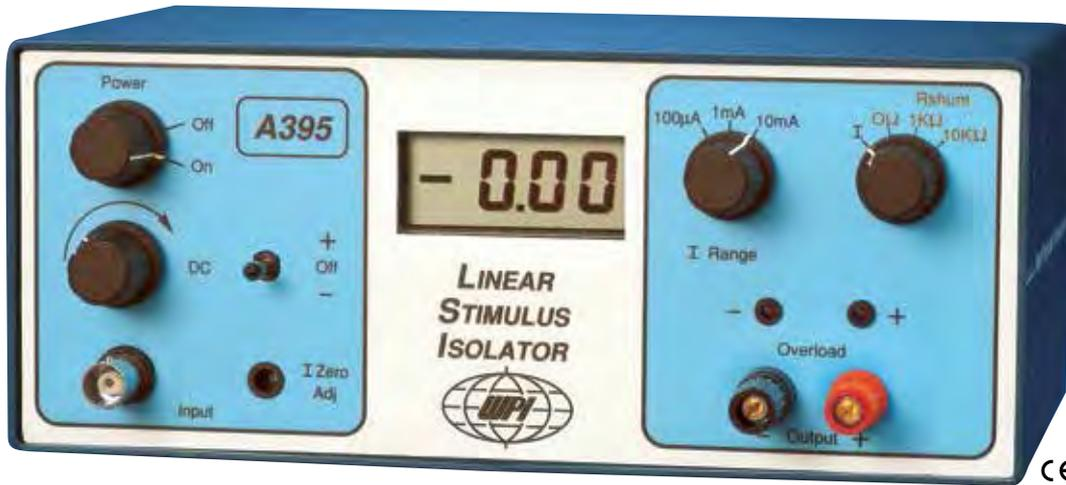
**Current Delivery** — A 10 V input produces the maximum output current for the current range selected, i.e., 100  $\mu$ A, 1 mA, or 10 mA. Front panel controls allow DC current to be generated. Externally applied signals can be superimposed simultaneously (DC offset). Warning lamps indicate open circuit or excessive current conditions.
