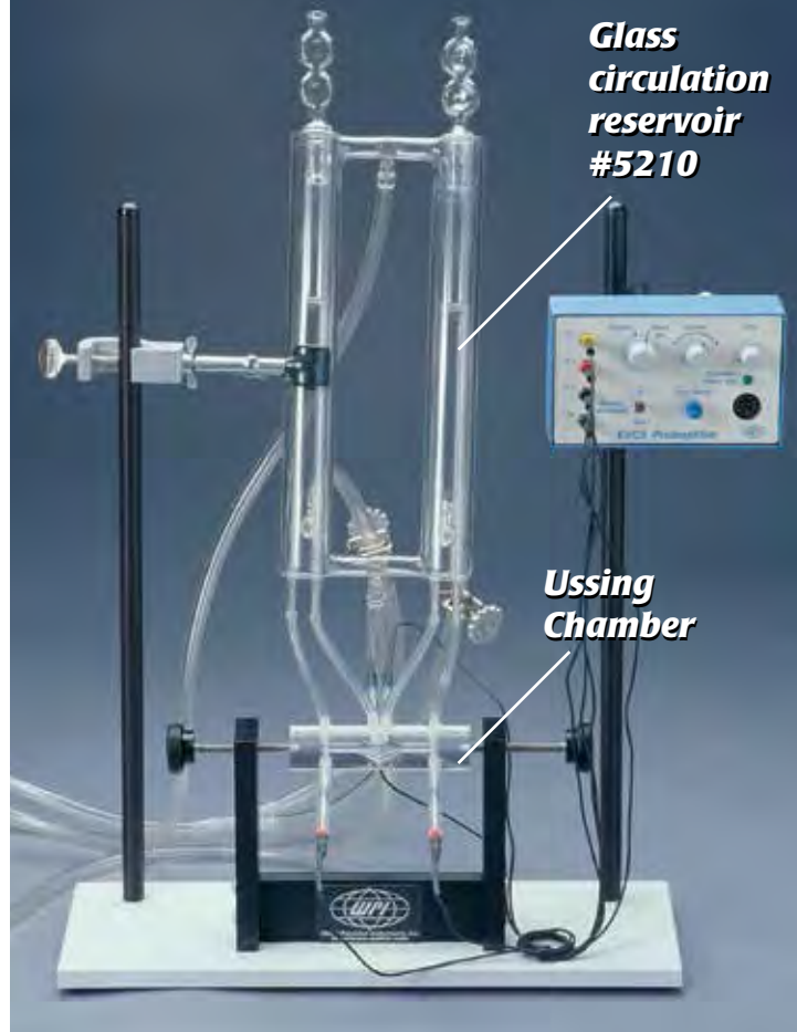
Complete Ussing System includes stand, glass reservoir, electrodes, Ussing chamber and tubing (EVC3 preamp and post mounting kit not included—see page 18).
