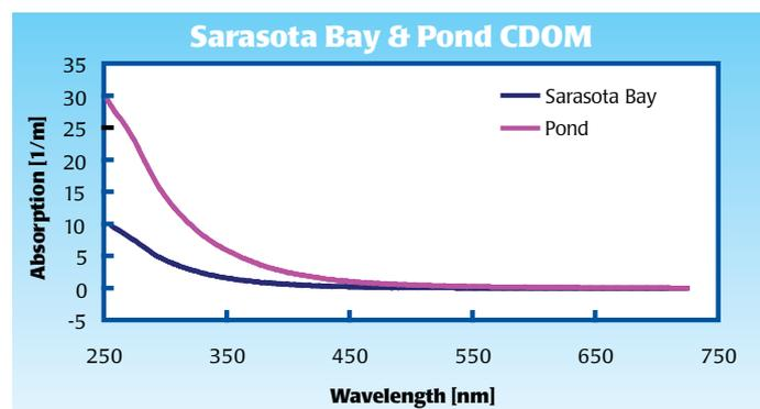
**Fig. 1** — Two typical absorption spectra measured using UltraPath. The sample labeled "Sarasota Bay" is a CDOM sample with 34 PSU salinity collected from Sarasota Bay (Nov. 2007), and the sample labeled "Pond" is a highly concentrated CDOM sample collected from a local pond in Sarasota, Florida (Nov. 2007).
