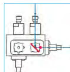
From the internal light source, radiated light passes through the cuvette holder and illuminates through the external measuring cell. The light is redirected through the cuvette holder and channelled through the detector.
