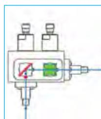
The light radiates from the internal light source, and is conducted from the redirected mirror, through the cuvette holder, into the correct detector. The measuring sample can be located in the second cuvette chamber.
