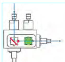
The light from the external light source is coupled over the cuvette holder and redirected over the mirror cuvette to the detector; thereby the sample in the standard cuvette chamber can be measured.
