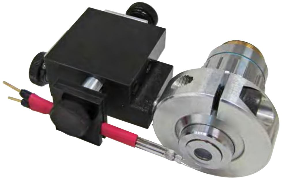
**Filament Holder mounts directly to objective to provide precise control of heating element position.**
